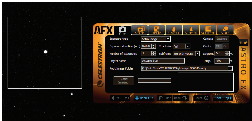
FIGURE 5: SELECTING THE SUBFRAME AREA
